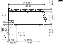
EQ = Equipotential screwG = Gas connection
